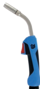
TBi 250 Classic Series 60% (10 min.) Mix: 200 A CO 2 : 230 A Ø 0.8-1.2 mm
