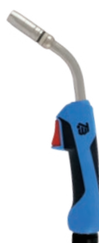
TBi 351 Classic Series 100% (10 min.) Mix: 270 A CO 2 : 300 A Ø 0.8-1.2 mm
