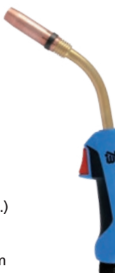
TBi 360 Classic Series 60% (10 min.) Mix: 300 A CO 2 : 330 A Ø 1.0-1.6 mm
