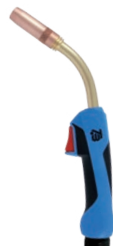
TBi 360 Classic Series 60% (10 min.) Mix: 300 A CO 2 : 330 A Ø 1.0-1.6 mm
