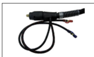
Rotating connection to govern welding wire feeder
